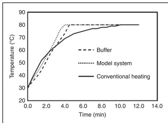
**Figure 1.** Temperature profiles of *Penicillium purpurogenum* GH2 pigment samples during ohmic and conventional heating treatments at 80 °C.
