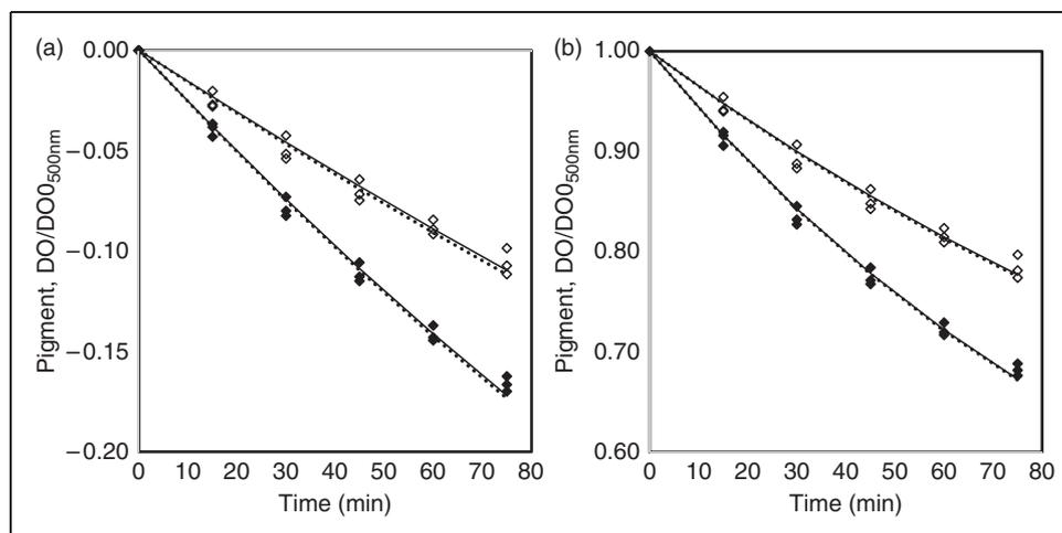
**Figure 2.** Color degradation kinetics of beverage model system processed by ohmic heating (◆) and conventional heating (◇) at 90 °C described by (a) Bigelow model and (b) first-order model. Full lines correspond to the fit of individual model and the dashed lines to global model.
