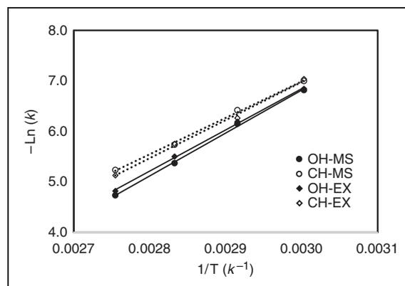
**Figure 3.** Diagnostic plot of temperature dependence given by the Arrhenius equation during ohmic heating (full lines) and conventional heating (dashed lines).
