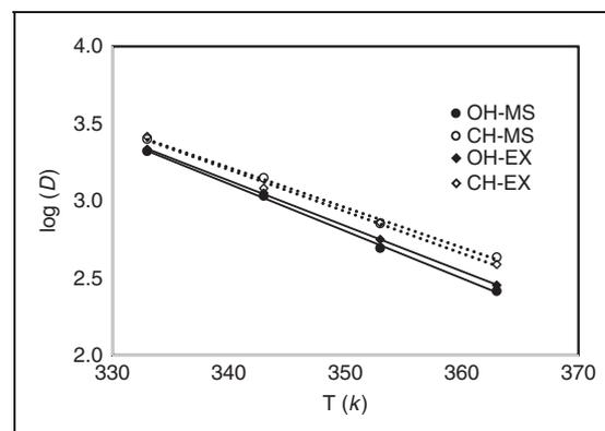
**Figure 4.** Diagnostic plot of temperature dependence given by the Bigelow equation during ohmic heating (full lines) and conventional heating (dashed lines).
