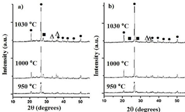
**Figure 2.** XRD patterns obtained for red ceramic bodies sintered using peak temperatures ranging from 950 to 1030 °C, with the addition of (in wt.%): a) 10% FA + 5% VE, and b) 10% MV + 5% VE. Key: ● Quartz ( $\text{SiO}_2$ ), ■ Anorthite ( $\text{CaAl}_2\text{Si}_2\text{O}_8$ ), and  $\Delta$  Hematite ( $\text{Fe}_2\text{O}_3$ ).
