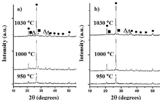
**Figure 3.** XRD patterns obtained for red ceramic bodies sintered using peak temperatures ranging from 950 to 1030 °C, with the addition of (in wt.%): a) 5% glass frit, and b) 5% FA + 1% C + 4% VE + 1%  $\text{Na}_2\text{P}_3\text{O}_{10}$ . Key: ● Quartz ( $\text{SiO}_2$ ), ■ Anorthite ( $\text{CaAl}_2\text{Si}_2\text{O}_8$ ), and  $\Delta$  Hematite ( $\text{Fe}_2\text{O}_3$ ).
