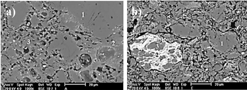
**Figure 4.** SEM micrographs obtained for a red ceramic body sintered using a peak temperature of 1000 °C, with the addition of: a) 10% FA + 5% VE (in wt. %); key: zone 1, quartz; zones 2 and 3, anorthite and hematite; b) 5 wt.% glass frit; key: zones 1 and 3, quartz; zones 2 and 4, anorthite and hematite.
