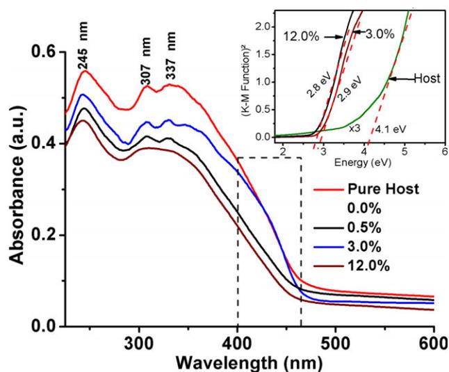
**Figure 3.** Absorbance spectra of the  $\text{Sr}_4\text{Al}_{14}\text{O}_{25}:\text{Eu}^{2+}, \text{Dy}^{3+}$  powders with different Bi concentrations and that of the pure host without dopants. The inset shows the Kubelka–Munk (K–M) functions *versus* energy for the pure host (without dopants), 0.0% Bi and 12.0% Bi-doped samples, the energy gap ( $E_g$ ) of the samples was calculated by intersecting the linear part of those curves with the axis of energy.
