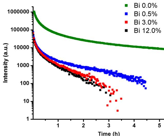
Figure 5. Curves of Phosphorescent intensity versus time for Bi-doped samples.
