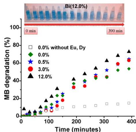
Figure 7. Degradation curve of methylene blue as a function of time under UV irradiation at 365 nm.
