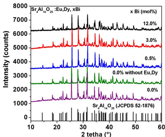
**Figure 1.** XRD patterns of the host sample (without dopants) and the  $\text{Sr}_4\text{Al}_{14}\text{O}_{25}:\text{Eu}^{2+}, \text{Dy}^{3+}$  phosphors doped with different Bi concentrations.
