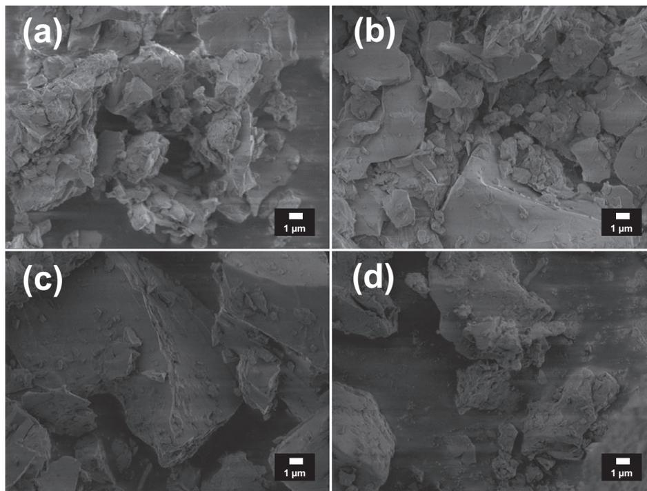
**Figure 2.** SEM images of: (a)  $\text{Sr}_4\text{Al}_{14}\text{O}_{25}:\text{Eu}^{2+}, \text{Dy}^{3+}$  phosphors (host without Bi) and Bi-codoped phosphors: (b) 0.5 mol%, (c) 3 mol% and (d) 12 mol%.
