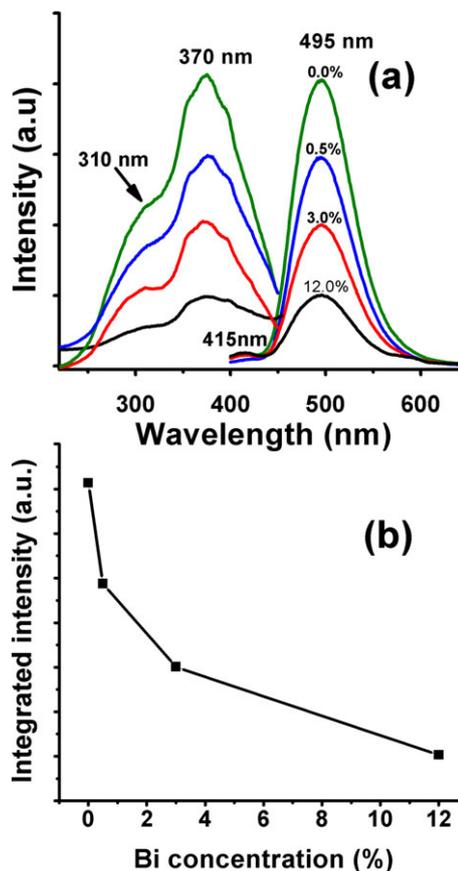
**Figure 4.** Excitation and emission spectra of powders with different Bismuth concentrations.
