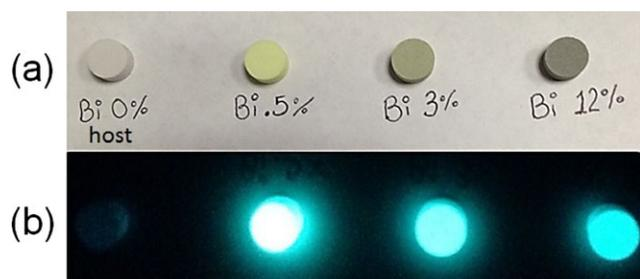
Figure 6. Pictures of the samples under (a) natural light (b) in darkness after 5 min of irradiation with the UV lamp (365 nm).
