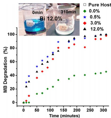
Figure 8. Degradation curve of methylene blue as a function of time under solar exposure in a sunny day in Saltillo City.
